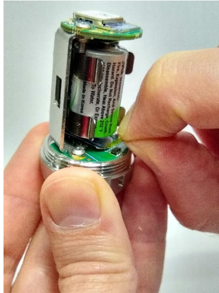
Figure 2: Battery Insulator Removal
