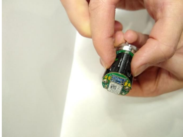
Figure 21: Clasp the Support by the Snap Arms with Thumb and Index Finger
